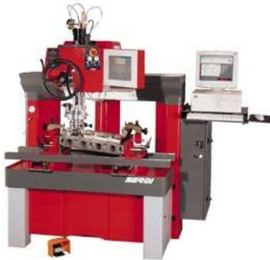
The **work head** of the machine is also under **numerical control**, allows automatic movement from one seat to another, giving a **complete machining cycle** for a given type of seat.
