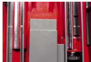
Axes mounted on guiding rails fitted with pre-loaded driving system through ball screw
