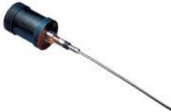
The EMP7 utilises ISE technology. Each particle travelling through the process develops an electrical charge. As the particle passes or impacts with the sensing element, a current is induced which is processed in EMP7 by a method called Impulse Signature Extraction ("ISE").
