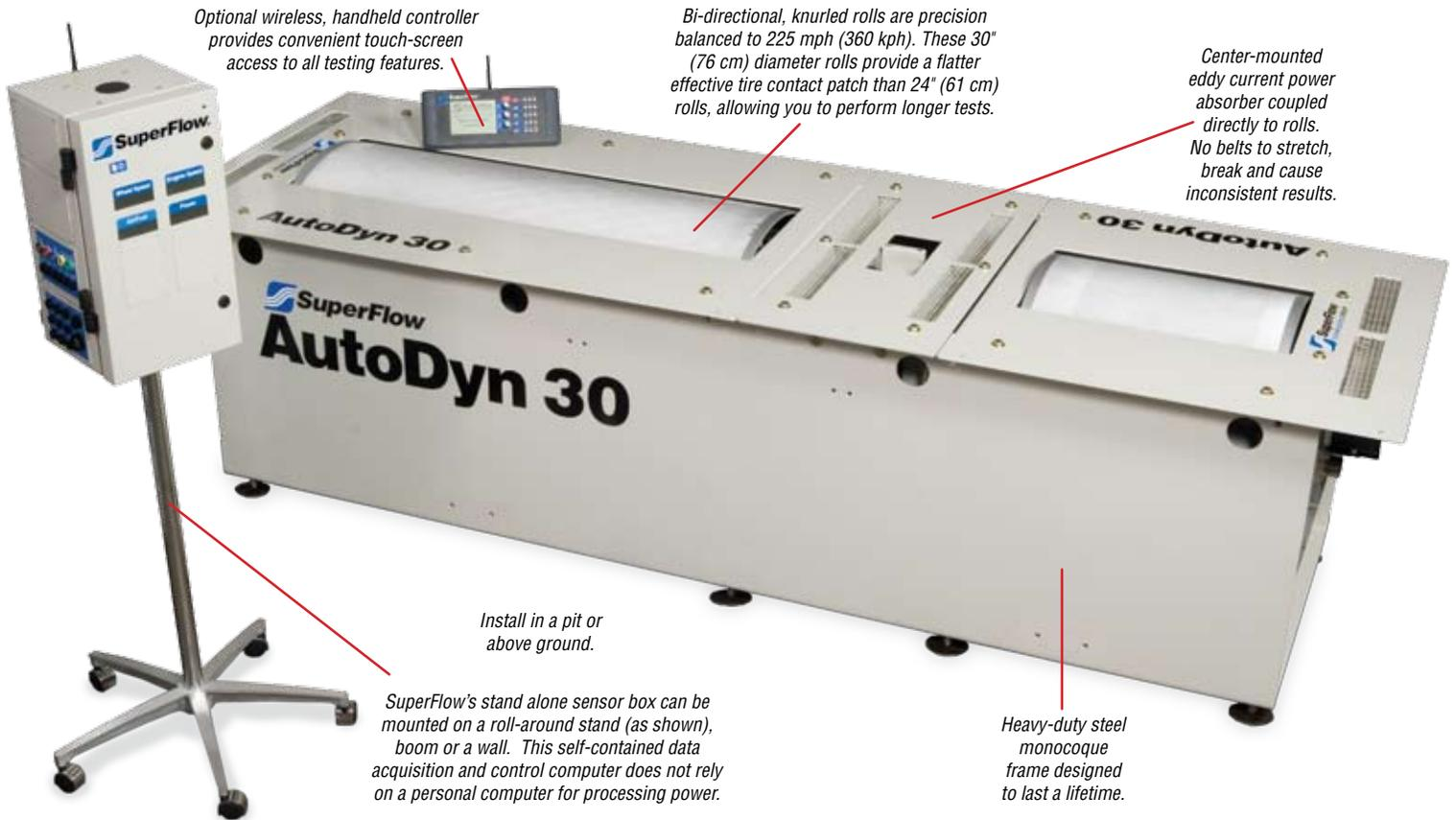
Optional wireless, handheld controller provides convenient touch-screen access to all testing features.
