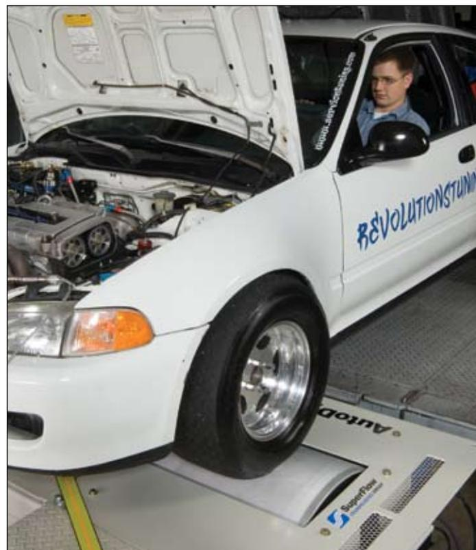
*Imports like this 600 hp turbocharged Honda CX hatchback rapidly find their way onto the new AutoDyn 30. Loading most vehicles is fast and easy. Large 30" (76 cm) diameter rolls provide ample surface area for this 600 hp Honda to apply its power.*
