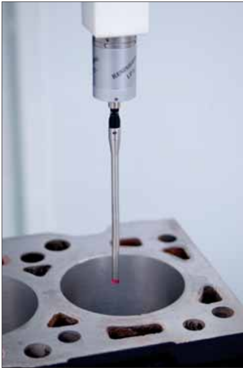
The electronic probe "Renishaw"
