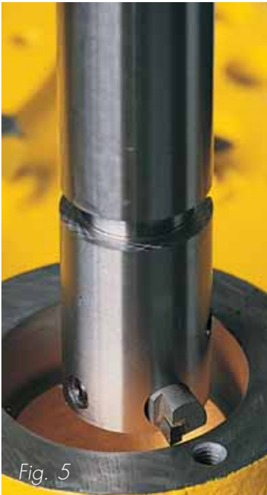
Fig. 5 - Boring a machine tool component with a dead-end hole tool.
