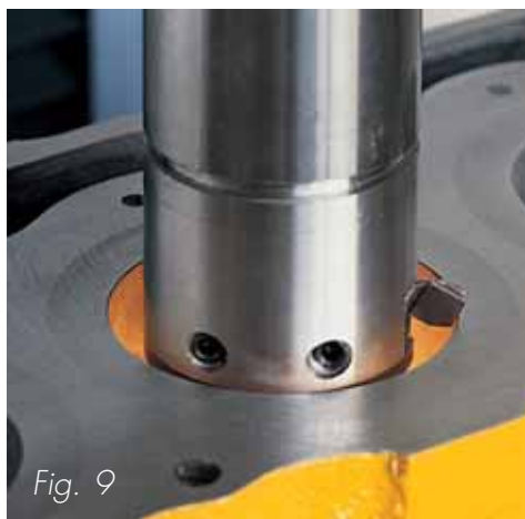
Fig. 6 - Centering a cylinder with the fixture equipping the boring spindle.
