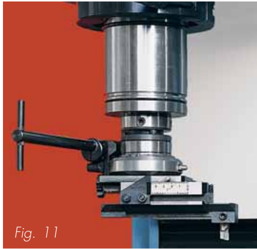
Fig. 11 - Toolhead with radial tool feed. Quite necessary for facing, milling and boring of counterbores.
